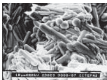
Figure 2.- SEM micrograph of \gamma' -Bi 2 MoO 6 pellet sintered at 900°C in air
